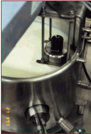
Fig. 4. Laboratory cheese vat fitted with combination of probes.
