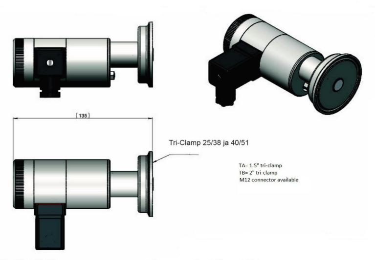
VOM with Tri-Clamp process connections, codes TA and TB
