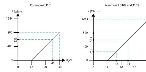
Figure 3: Intrinsically Safe Installations
