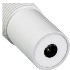
Figure 4 High performance (S) glass – flat with flush body
