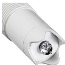
Figure 5 ORP electrode with notched body
